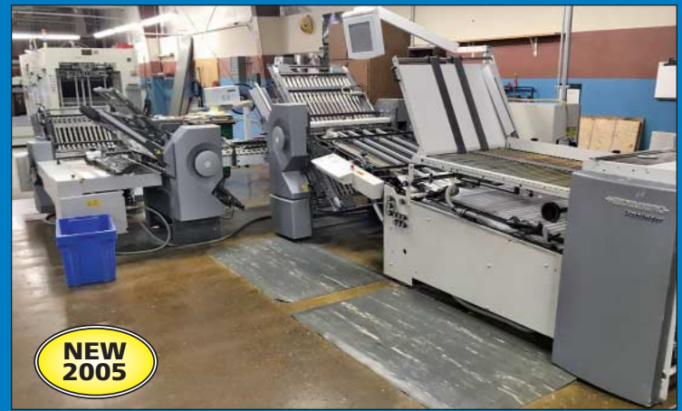
32" X 48" Heidelberg Stahl Model Model TH-82 6/4/4 Continuous Feed Folder
